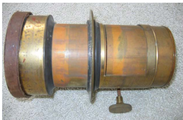
Fig. 10 Telephoto lens developed by Alexander McKay, and described in his 1890 paper. Private collection (photo: Hamish Campbell).
