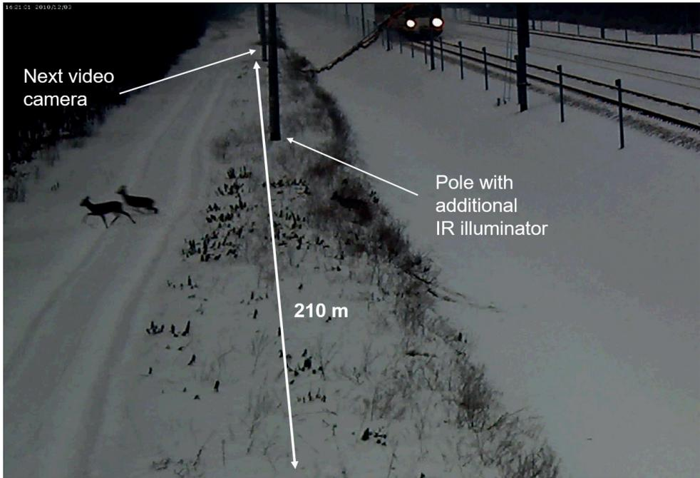
**Figure 4.** View from a digital camera set at the monitored stretch of E65 railway line, where wildlife warning reflectors were tested: an escape of two roe deer before an oncoming train is shown. The view from one camera extends beyond the pole with the next video camera to ensure that the whole stretch (marked with the white two-arrow line) is monitored.
