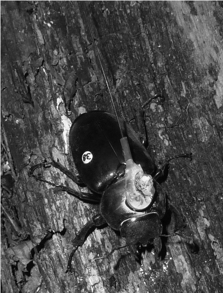
Figure 1. A female of Lucanus cervus marked with a numbered sticker on the right elytron and equipped with a battery-powered radio transmitter (LB-2X / 0.31g; Holohil Systems Ltd., Carp, Ontario, Canada).
