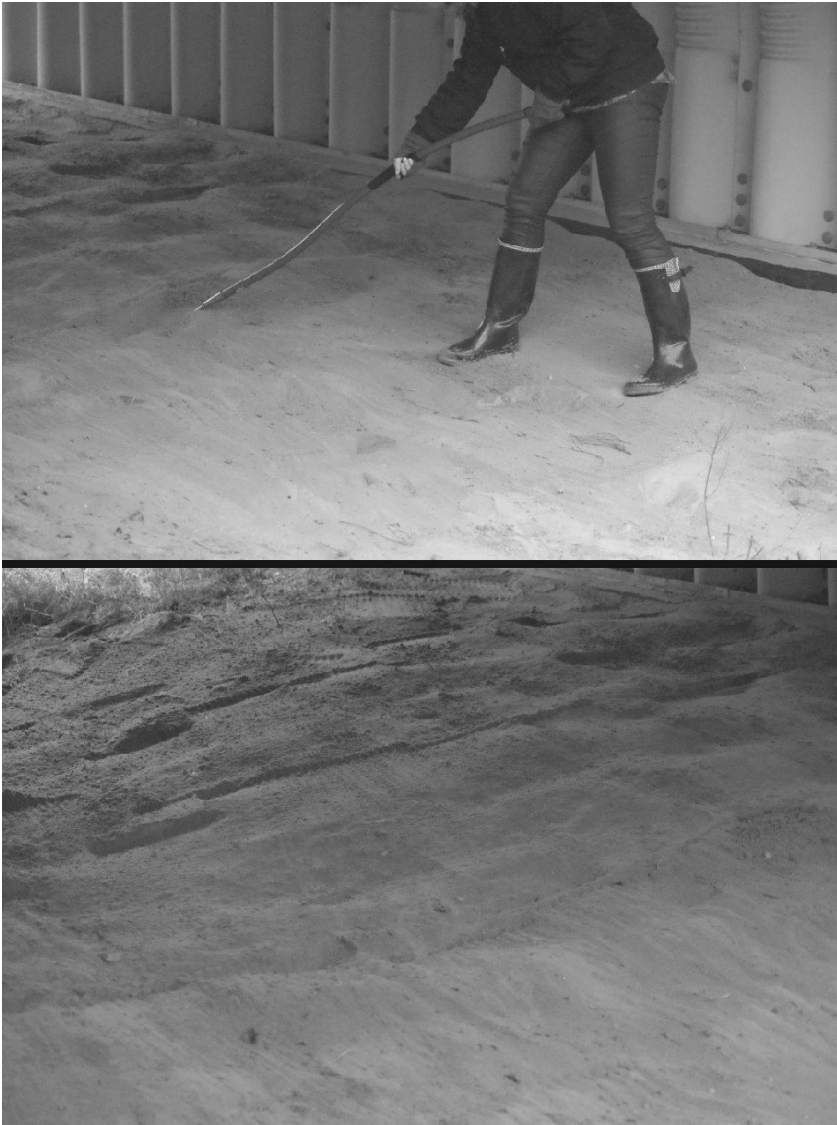
Figure 3. Preparation of track beds for survey of animals' activity in underpass in S3 expressway.
