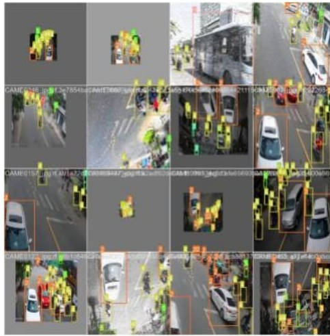
Figure 15: Testing the trained model by employing modified dataset images to simulate harsh weather conditions.
