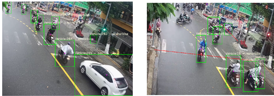
Figure 9: Different stages of traffic light. (1) On green light the system will halt its violation tracking. (2) The system resume violation detection on red-light
