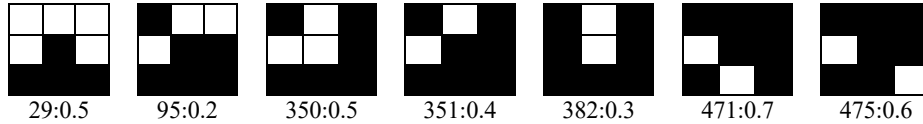
Figure 7: The tile-based representations of the seven successful 2D LCA environments with their initial state densities, where caption xxx:y.yy indicates the tile for rule number xxx with initial density y.yy
