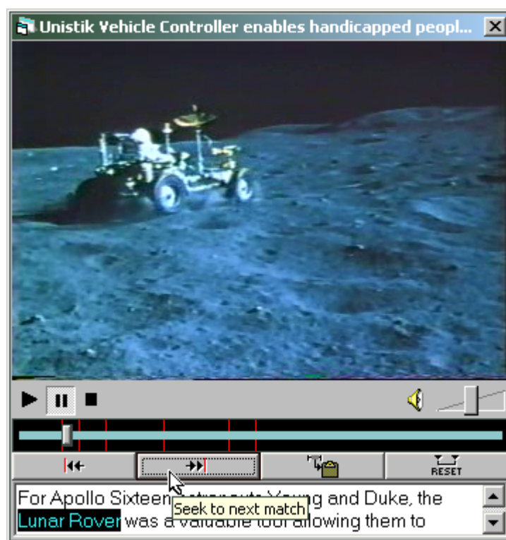
Figure 1: Effects of seeking directly to a match point on "Lunar Rover", courtesy of tight transcript to video alignment provided by automatic speech processing.
