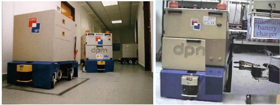
Figure 1: Left: The ARIADNE-team: Odysseus, Marvin, and Thor executing service orders. Each robot is equipped with four drawers, two on each side. Right: A robot automatically charges its batteries.
