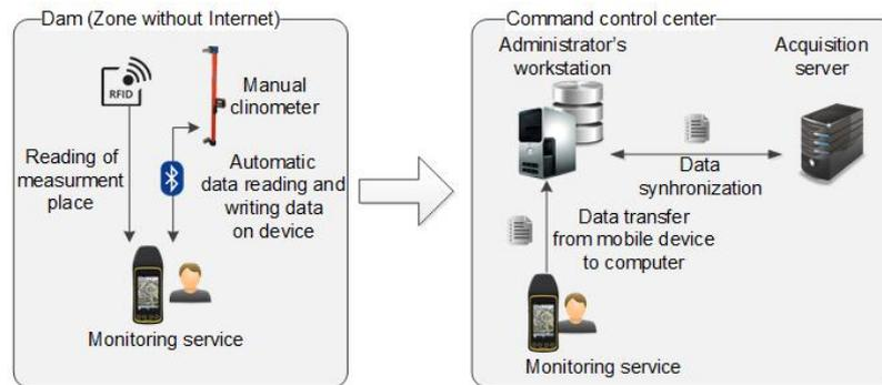
Figure 3: Model of the improved dam monitoring system
