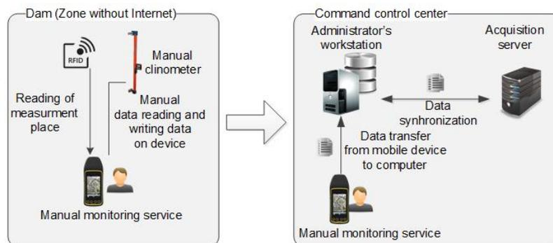
Figure 2: Manual dam monitoring system diagram
