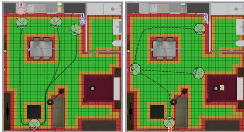
Figure 4: Test tasks (top view of the scenario). Task 1 (left): it consists of reaching the bottle of water dashed in blue (1), the oilcan in yellow (2) and, finally, the cake box in red (3). Task 2 (right): it consists of reaching the refrigerator dashed in blue (1), the bed in yellow (2) and the window in red (3). The ideal paths to reach each of the targets are shown with dashed lines.
