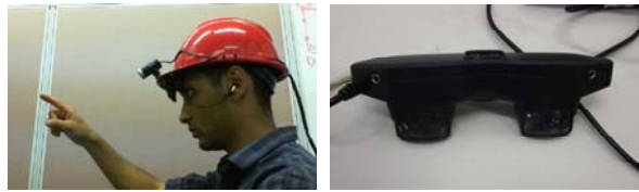
Figure 1: Helper performs gestures in the air (left) and the near-eye display (right)
