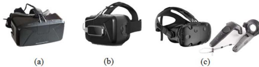
Figure 3: The three types of devices used in the first experiment: (a) the Oculus RIFT DK2; (b) the Oculus RIFT DK2 with Leap Motion tracker; and (c) the HTC Vive headset with its Dual-Handle controller.
