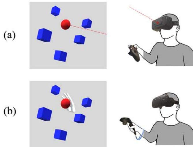
Figure 9: The technique using scenarios in Experiment 2: (a) RayCasting; (b) Virtual Hand.
