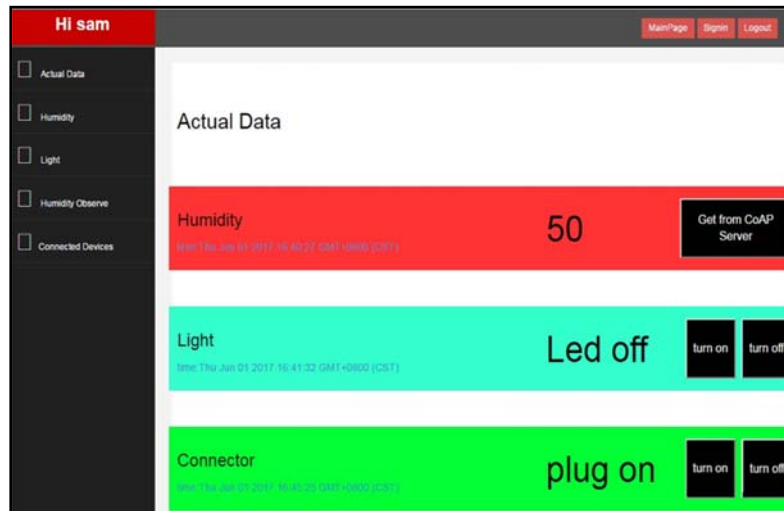
Figure 15: Web interface connected to the web server at 6LBR 1
