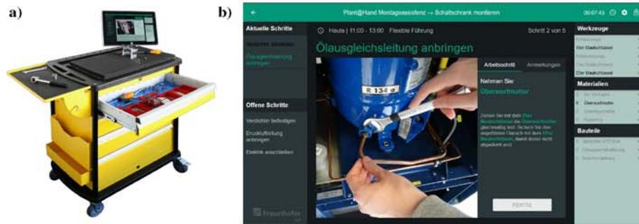
Figure 1: The Plant@Hand assembly assistant by Fraunhofer IGD: a) An assembly trolley is equipped with an assistance system [Alm et al. 2015b]. b) The display at the work station shows information supporting the current work task.
