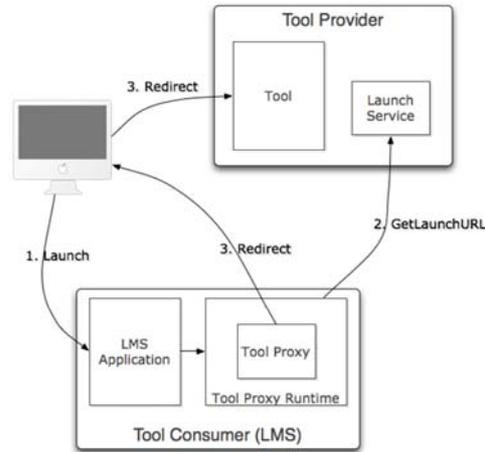
Figure 2: BLTI Launch process diagram.
