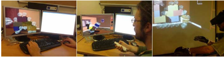
Figure 5: InputSubsystems used in the prototype: using mouse and keyboard; using the Wiimote device, and using data gloves and trackers.
