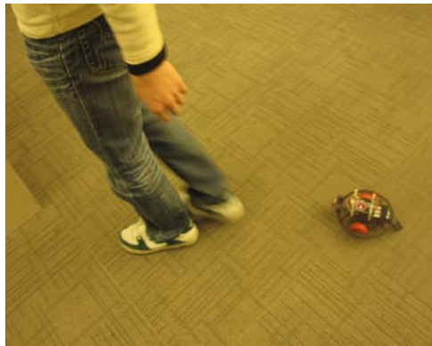
Figure 3: Human following with infrared sensing and servo control
