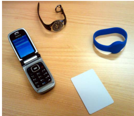
Figure 1: Mifare Standard 1K and 4K tags and Nokia NFC 6131 used in the evaluation.
