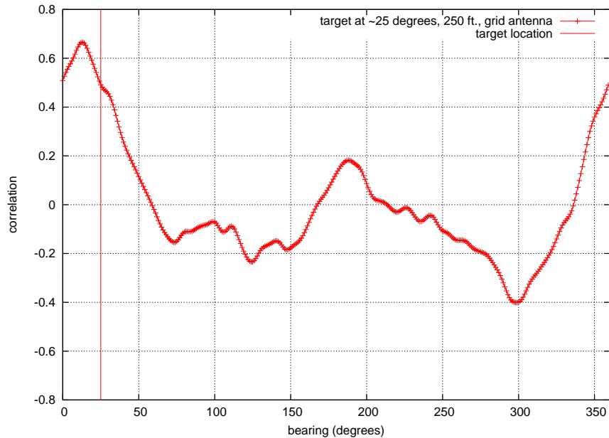
Figure 5: Correlation values of the May 9 grid antenna trial with the April 11 training data; the maximum correlation occurs at 13°.
