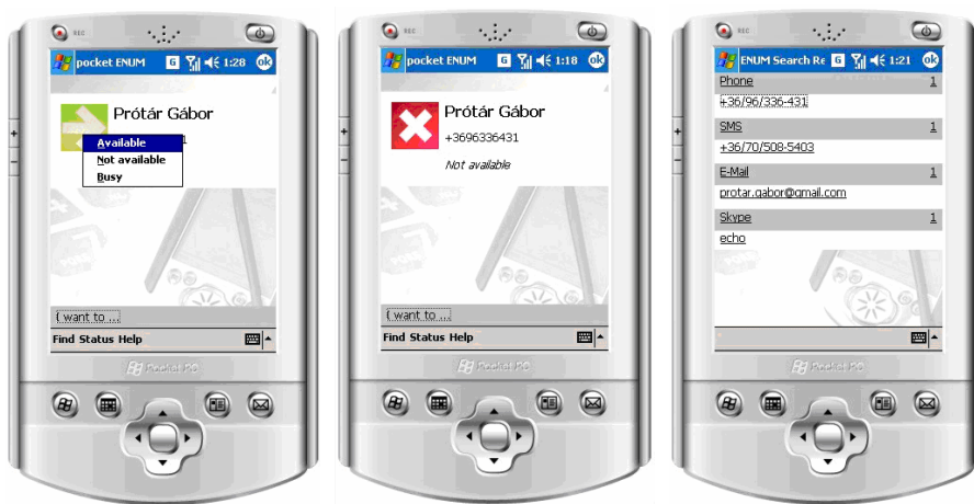
Figure 4: Screens of PocketENUM mobile application: (from left to right) Changing the actual state, Displaying the state, Making a query
