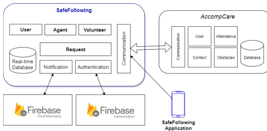
Figure 2: The SafeFollowing architecture
