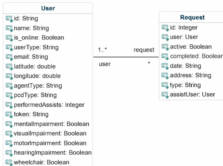
Figure 3: The SafeFollowing class diagram
