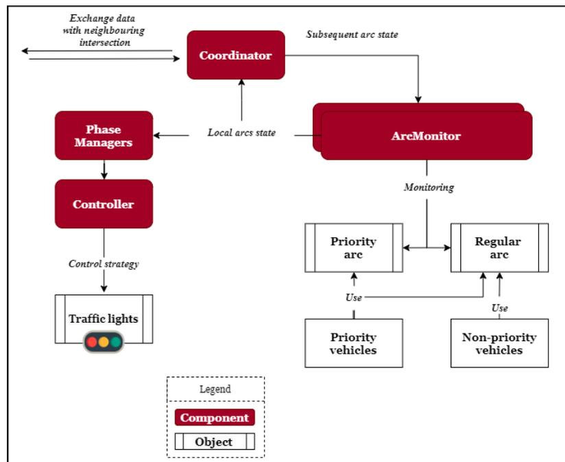
Figure 2: the components of the generic TSCS
