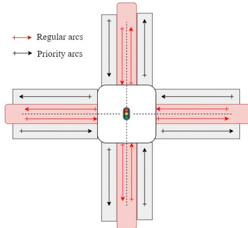
Figure 1: Intersection between two ordinary roads and two priority roads
