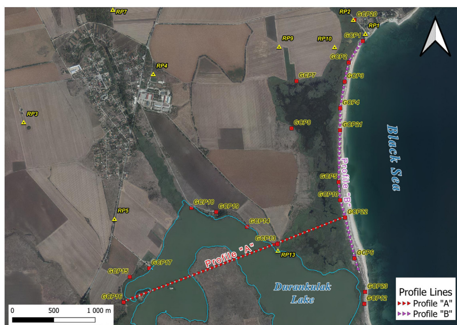
Figure 7. Profile lines used for comparisons of the four DEMs. GNSS control points (GCP) are marked with red squares, and geodetic reference points (RP) are marked with a yellow triangle.
