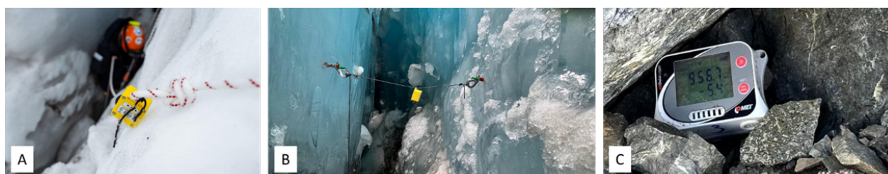
Figure 2. Sensors on site A and B sensors for air temperatures in crevasses of Johnsons Glacier C outside meteo data loggers Comet U4130.
