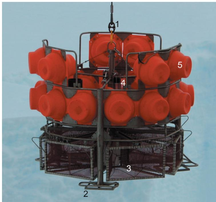
**Fig. 1.** Fish trap with (1) a hook for deploying and recovering the device and (2) feet, on which a set of weights (350 kg in total) are attached to keep the trap on the seabed after the deployment. Bait was placed into the creels (3) to attract the fish. An acoustic signal induces the detachment of the fish trap from the weights by the reloser (4) and its rise to the surface by means of several floats (5)
