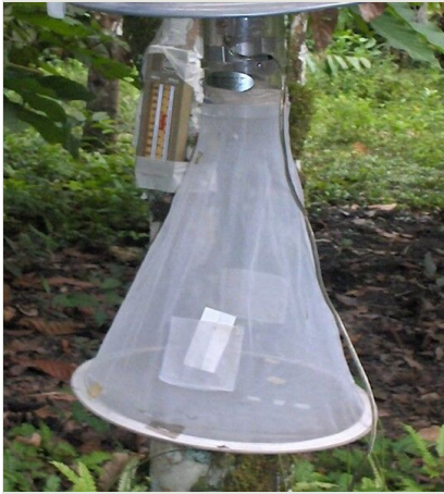
Figure 3. Light traps for the capture of Culicoides spp.
