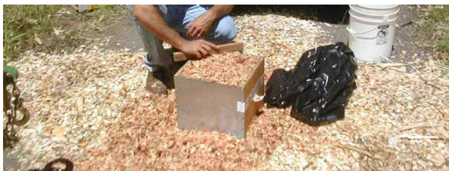
Figure 2. Measuring wood chips bulk density in Hawaii, USA (Turn et al. 2005)
