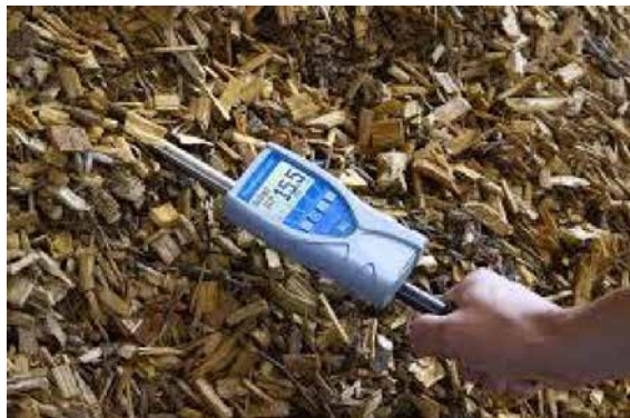
Figure 5. Measuring moisture content of wood chips in Australia (Boucher, 2019)
