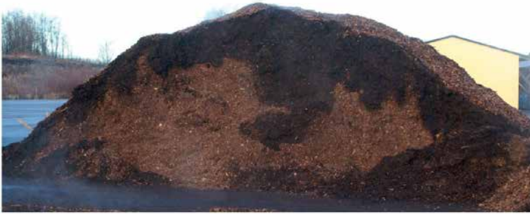
Figure 4. Uncovered cross section of wood chips pile in Sweden (Wästerlund et al. 2017)
