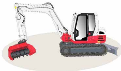
Fig. 5. Mini-excavator for mechanical mastication treatment in the USA (Becker and Keffe, 2020)
