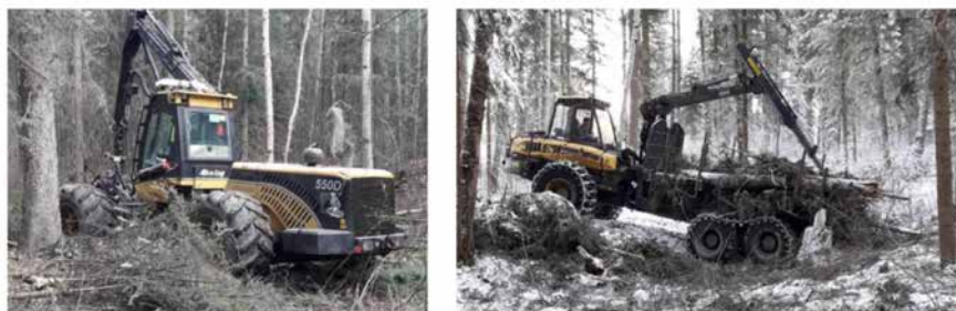
Fig. 1. Harvester and forwarder application in thinning to reduce fire risk in Canada (Dyson and Hvenegaard, 2021)
