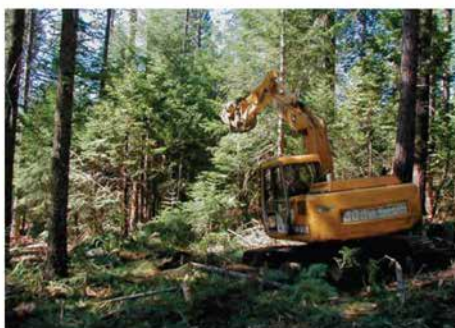
Fig. 4. Rotary masticator operating in mixed forests in California (Stephens et al. 2012)
