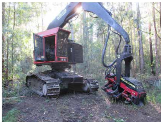
Fig. 7. A harvester applied in mechanical fuel load reduction trial in Australia (Acuna et al. 2018)
