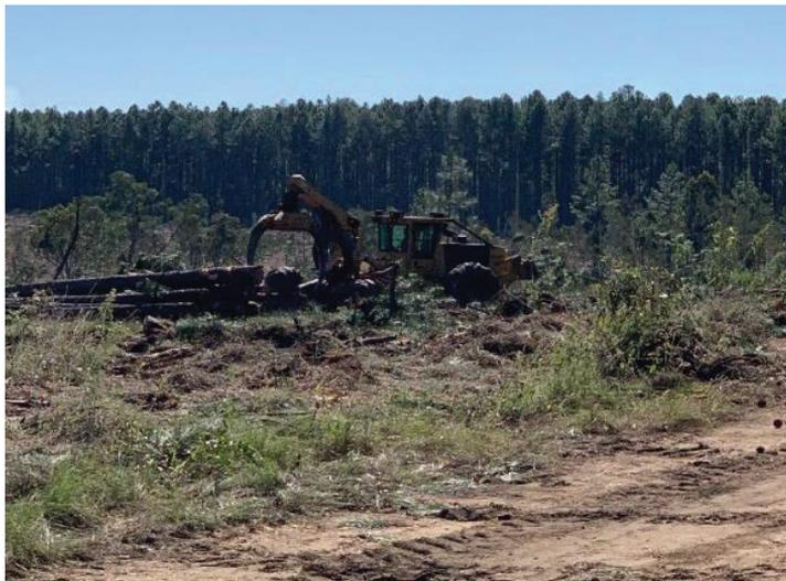
**Figure 1.** Grapple skidder working in pine plantations (Queensland, Australia)
