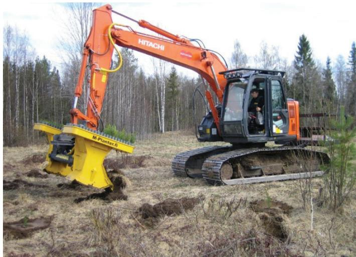
**Figure 1.** M-planter based on excavator in Finland (<http://www.m-planter.fi/en/M-Planter.html>)
