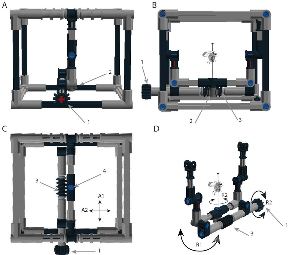
**Figure 2.** The IMp model shown from a side view (A), front view (B), top view (C) and without the stabilizing case exposing the pivot arm wherein the specimen is placed (D). Figure labels and abbreviations: pivot handle (1), 8 tooth gear (2), worm gear (3), connector peg that holds and rotates the specimen (4), axis of movement 1 (A1), axis of movement 2 (A2), axis of rotation 1 (R1) and axis of rotation 2 (R2).
