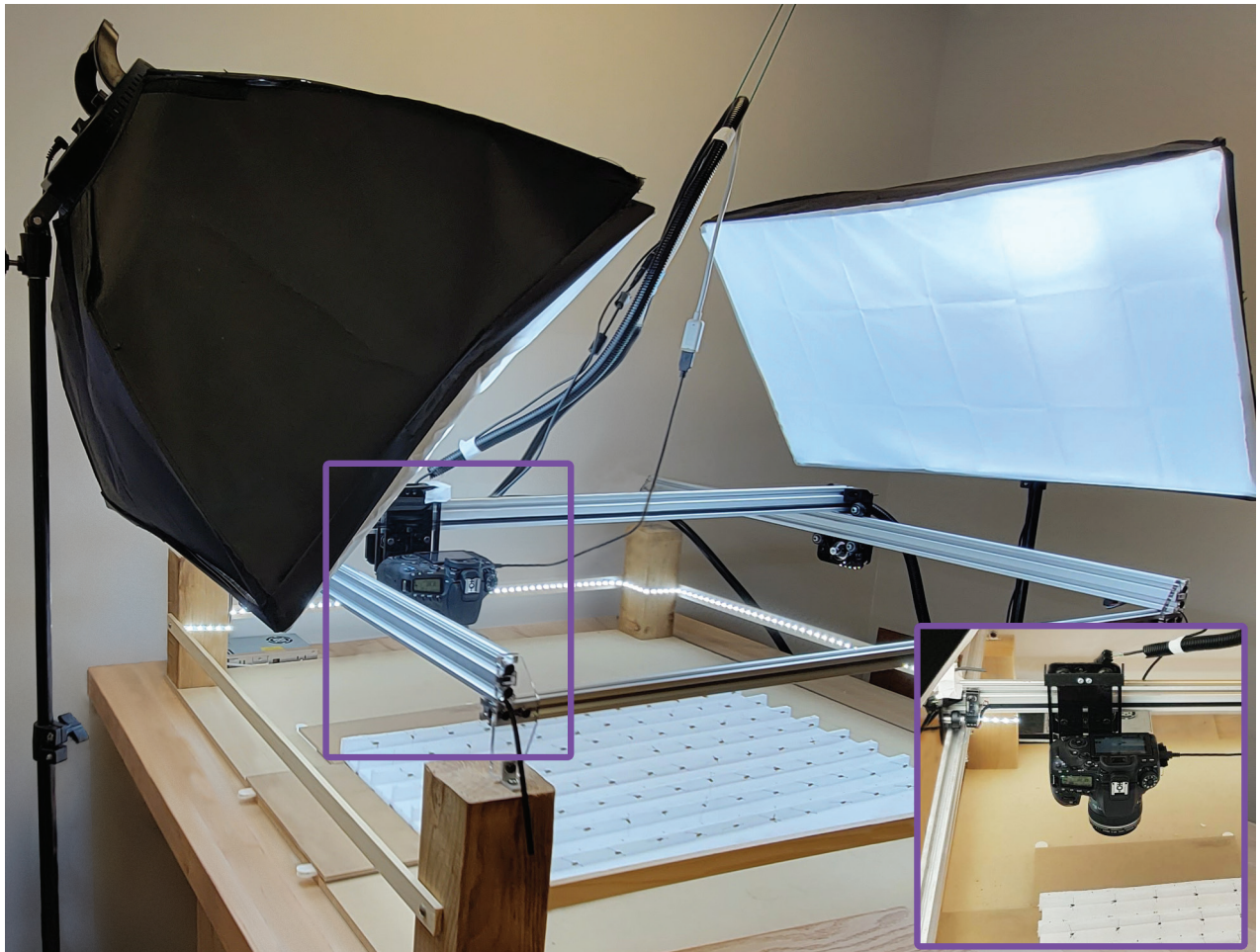
Figure 1. The SLR rig is placed on a heavy-base table to minimize vibration. The inset shows the actual rig area with specimens on the styrofoam base.
