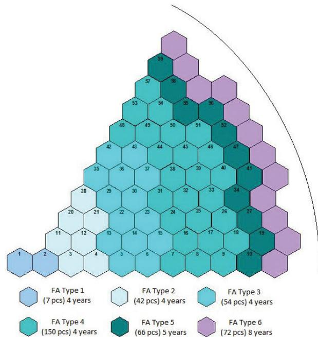
**Figure 1.** Reactor core map grid.
