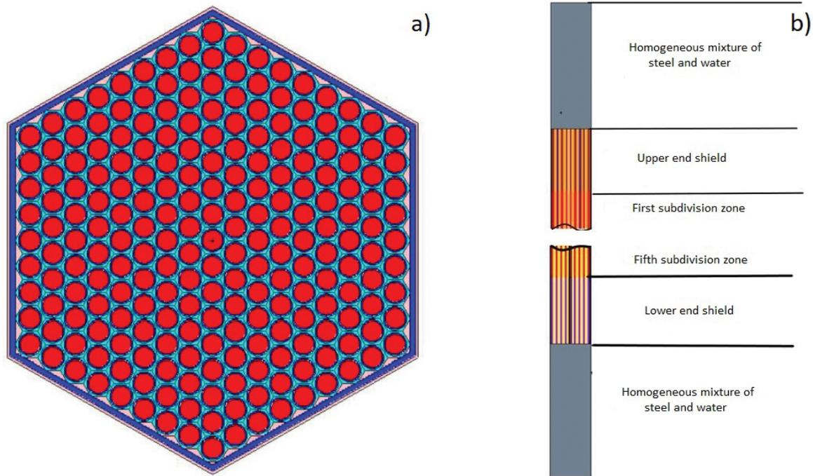
**Figure 2.** Fuel assembly calculation model: **a)** – horizontal projection; **b)** – vertical projection.
