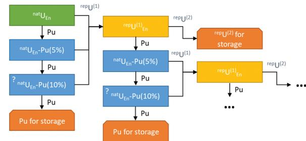
Figure 5. Nuclear material cross-utilization scheme.
