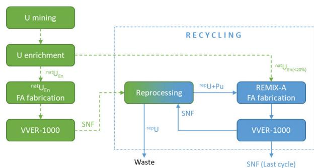
**Figure 1.** REMIX-A recycling scheme when  $^{235}\text{U}$  is enriched up to 20%.
