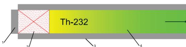
**Figure 1.** Computational model of the traveling wave reactor: 1 – absorber region; 2 – seed region; 3 – reflector; 4 – fertile material region.
