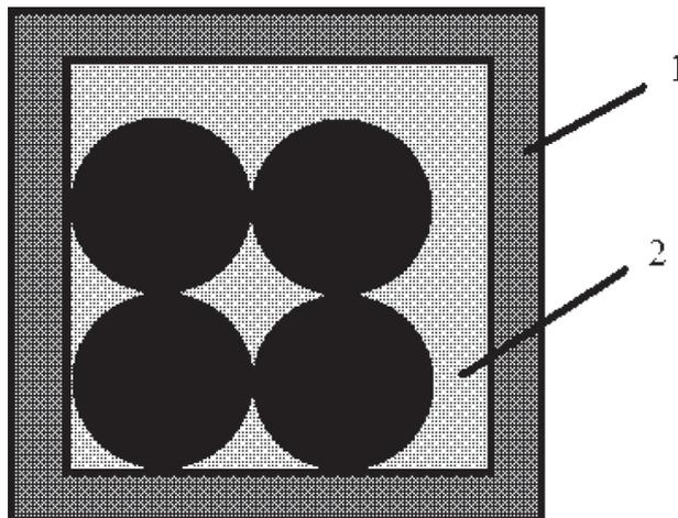
**Figure 1.** An example of the asymmetrical NZK-150-1,5P cask (secondary package) loading pattern: 1 – concrete cask wall, 2 – filler (extra biological shielding).
