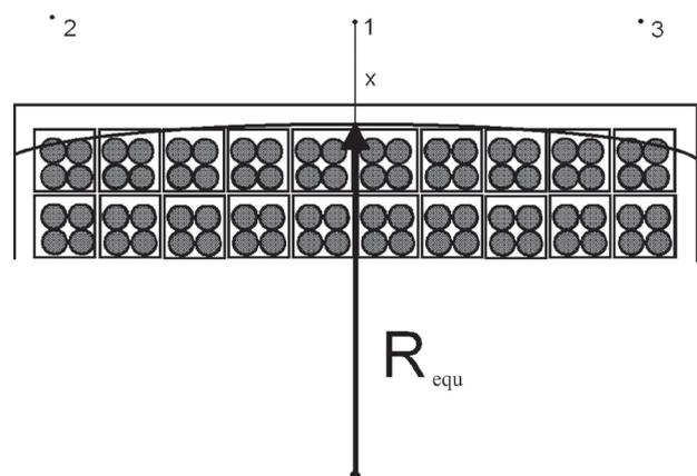
**Figure 4.** A model to assess the radiological situation around a hangar-type storage facility.
