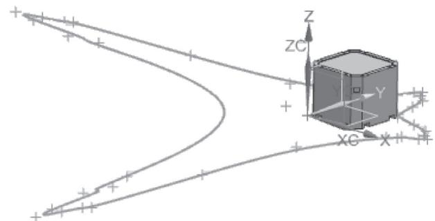
**Figure 6.** Software-predicted distribution of the gamma dose rate from a filled NZK-150-1,5P cask.
