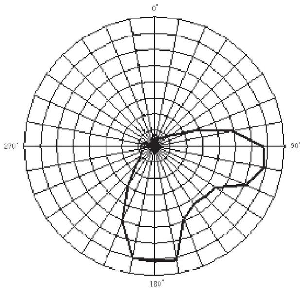
**Figure 2.** Directional pattern of gamma radiation from a filled NZK-150-1,5P cask.
