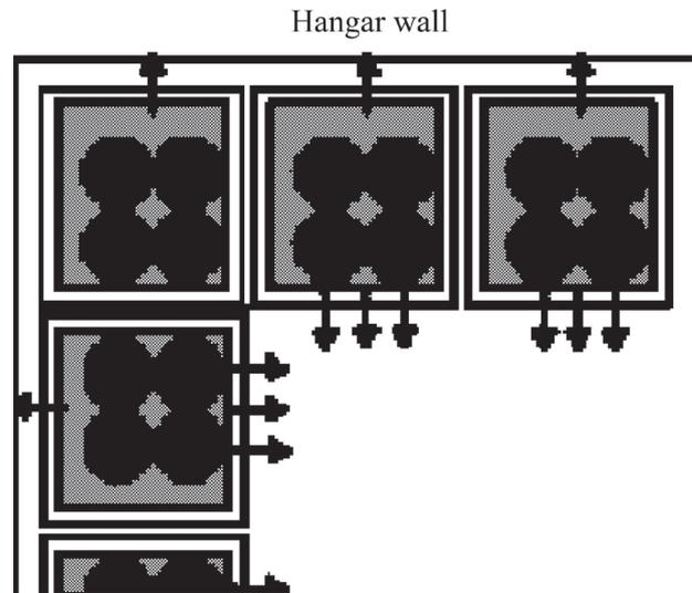
**Figure 3.** Diagram of the external cask orientation in the storage facility's peripheral rows.
