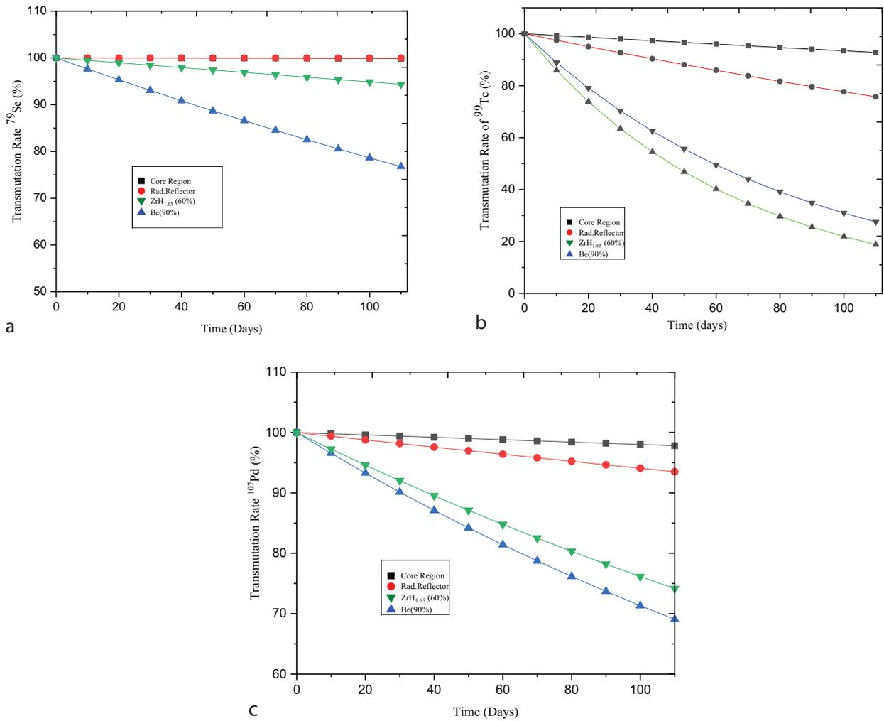
**Figure 5.** Transmutation rate evolution for <sup>79</sup>Se, <sup>99</sup>Tc and <sup>107</sup>Pd.
