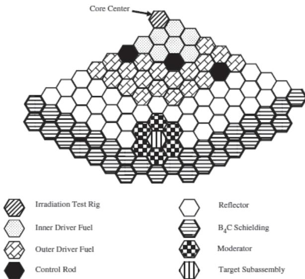
Figure 3. Target assembly location (1/3<sup>rd</sup> core configuration).
