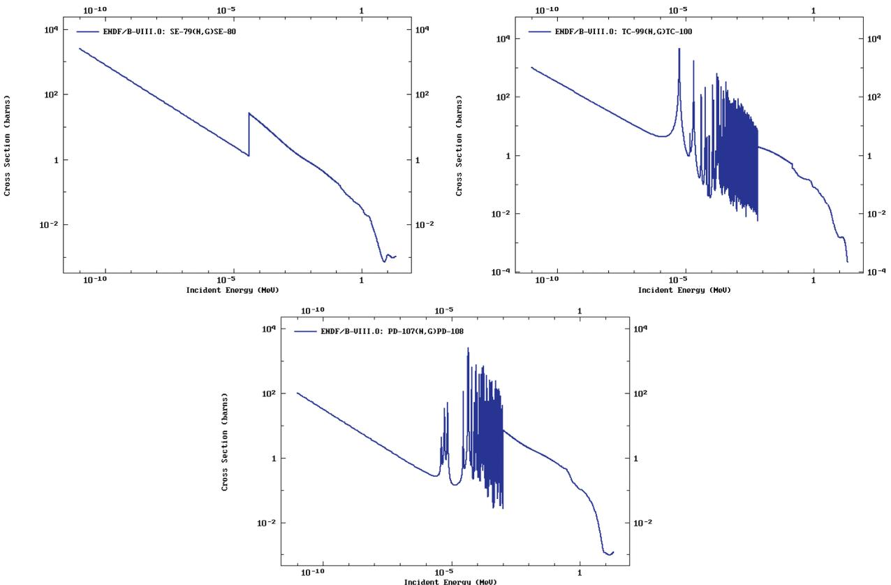
**Figure 4.** Neutron absorption cross section from ENDF file, (a)  $^{79}\text{Se}$ , (b)  $^{99}\text{Tc}$ , (c)  $^{107}\text{Pd}$ .
