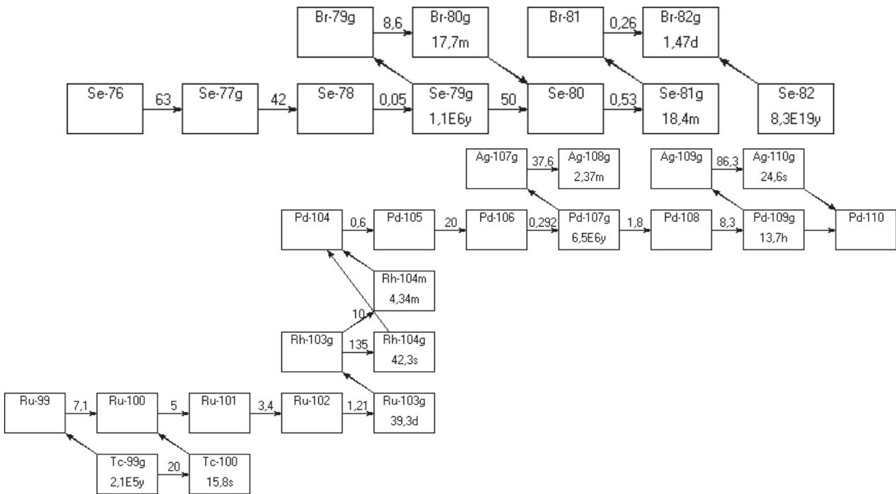
Figure 2.  $^{79}\text{Se}$ ,  $^{99}\text{Tc}$  and  $^{107}\text{Pd}$  transmutation chain under neutrons irradiation.
