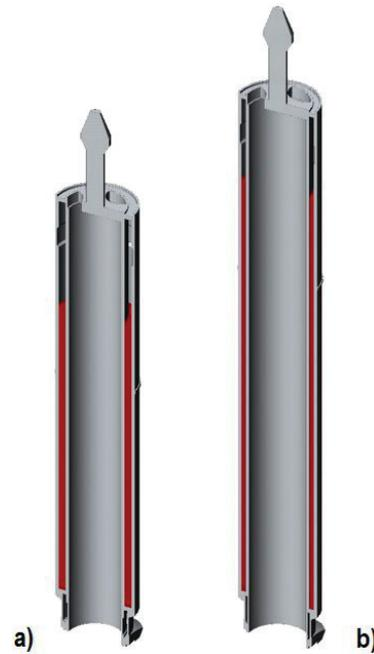
**Figure 3.** Comparison of targets: a) currently in use; b) upgraded.
