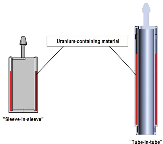
**Figure 2.** Targets used for the Mo-99 generation in the VVR-c reactor (vertical cut).
