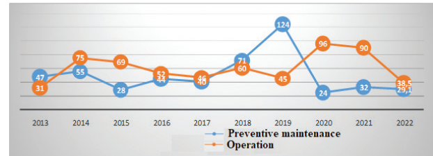
Figure 7. Solid RW formation at the ANPP in the operation and preventive maintenance periods, m 3 /year.
