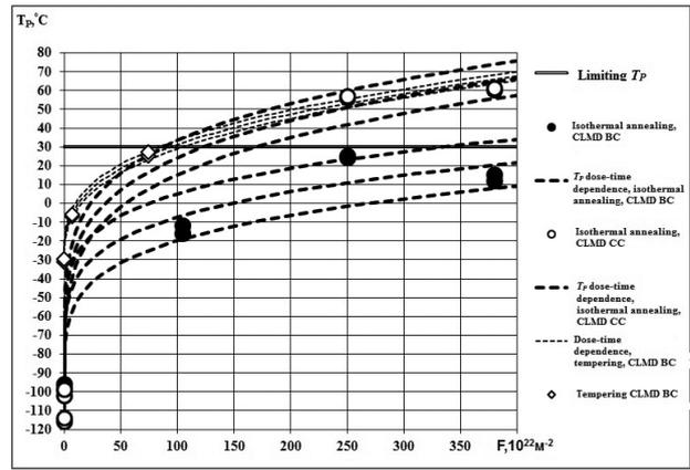
**Figure 3.** Dose-time relationships of  $T_p$  for the results of testing small-size impact testing samples made of experimental CLMD metal from commercial of KStK1 stock with base chemical composition subjected to standard “isothermal annealing” thermal treatment and “tempering” thermal treatment.
