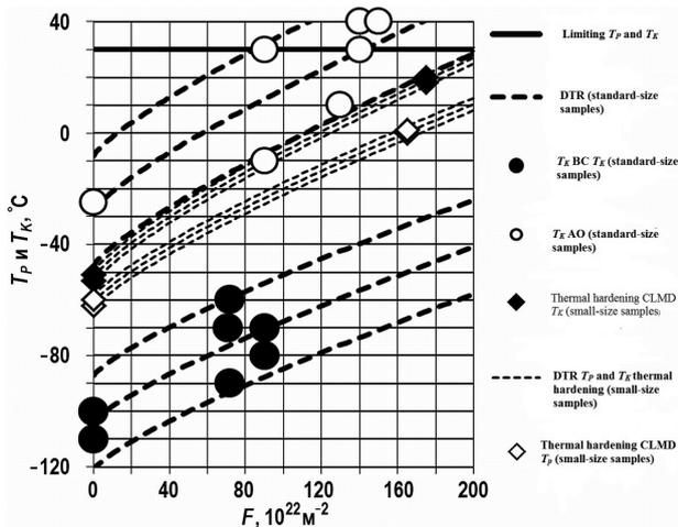
**Figure 1.** Dose-time relationships of  $T_K$  and  $T_p$  for the results of testing standard-size and small-size samples made of KStK1 with base chemical composition subjected to “thermal hardening” treatment.
