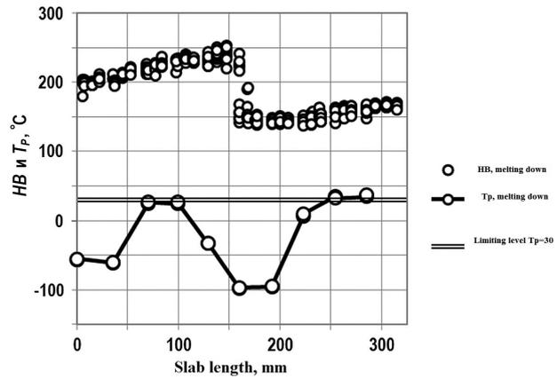
**Figure 6.** Distributions of hardness  $HB$  after additional equalizing melting down and  $T_p$  after melting down along the length of the process model of the weld fusion boundary between the base metal and the anticorrosive cladding metal before and after equalizing melting down.
