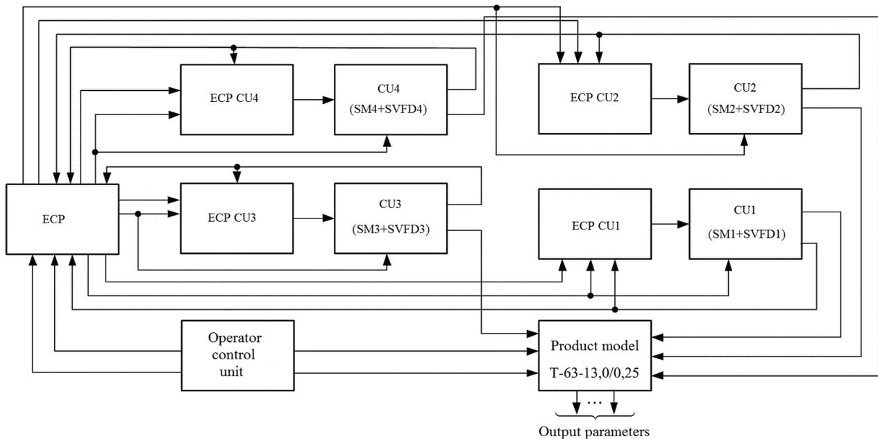
**Figure 1.** Functional diagram of the automatic control system for product T-63-13,0/0,25 (condensation mode).
