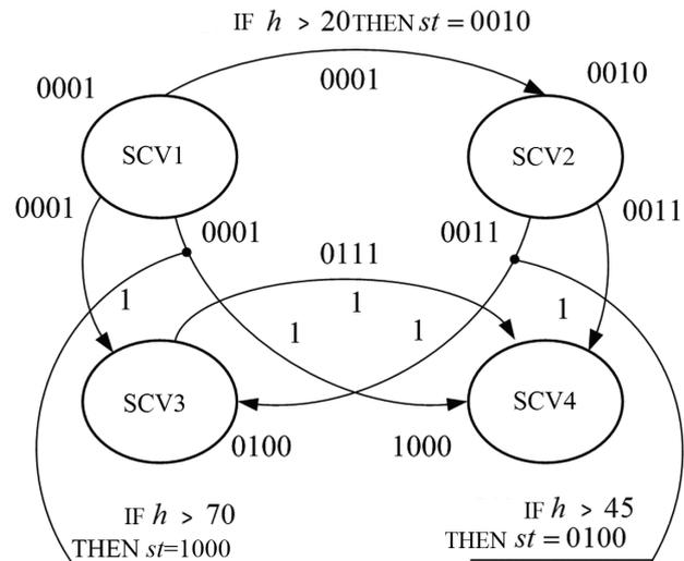
**Figure 7.** Constitutional diagram of control valves, SCV1 through SCV4, in control of steam supply to the T-63-13,0/0,25 ST.
