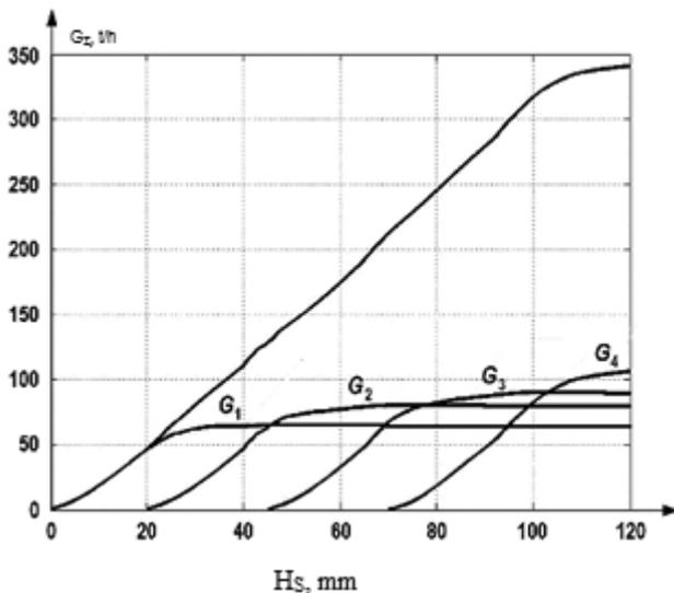
**Figure 6.** Diagrams of steam flows through the HPS control valves (SCV1 through SCV4) as a function of their strokes.
