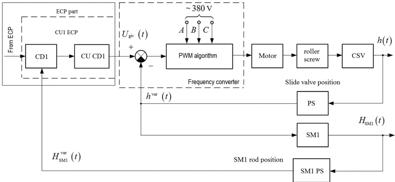
Figure 4. Functional diagram of the CU1 control unit with a control device (CU1 CD).
