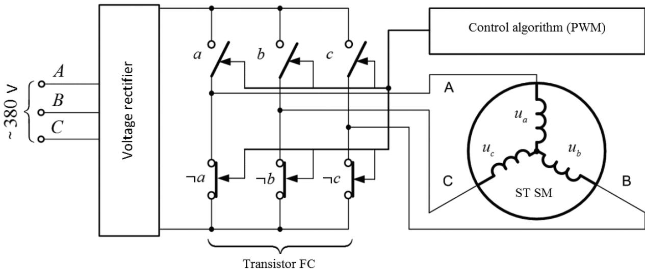
Figure 2. ST synchronous motor feed circuit.
