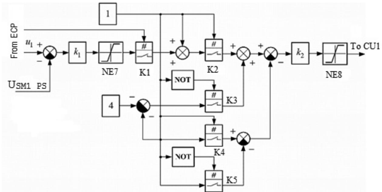
Figure 5. Block diagram of the control device for CU1 control unit.
