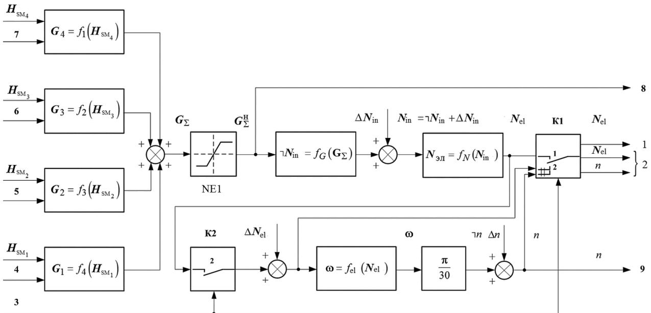
Figure 3. T-63-13,0/0,25 block diagram.
