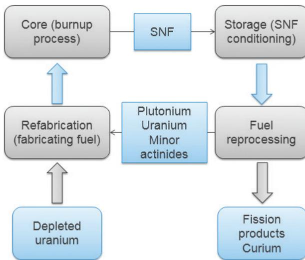
**Figure 1.** Diagram of the fuel cycle implementation in a lead-cooled fast reactor
