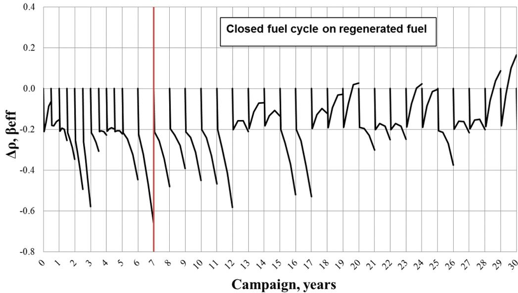
Figure 2. Time dependence of the reactor core reactivity change
