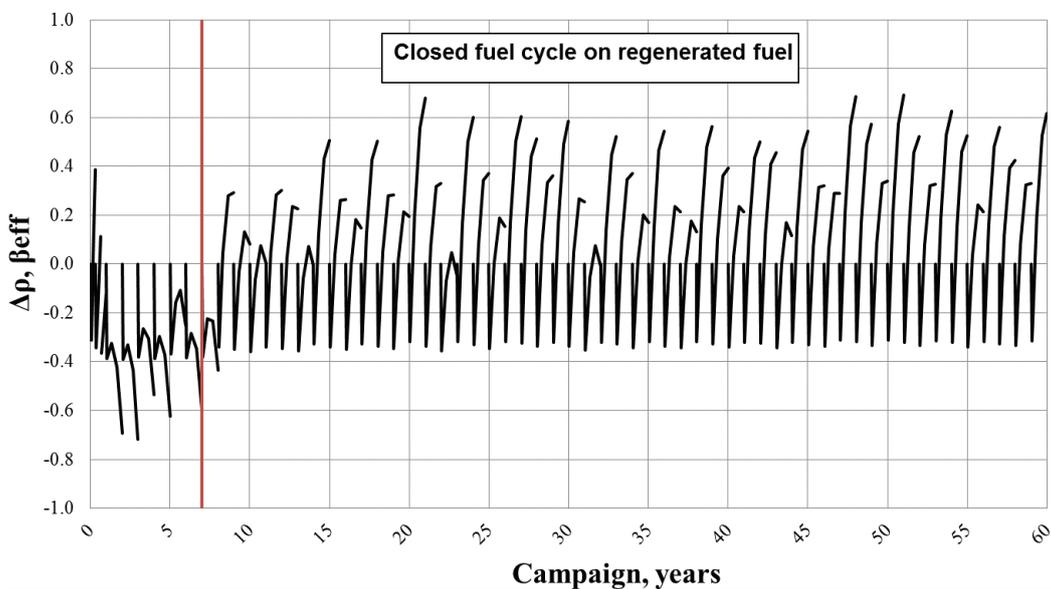
Figure 4. Time dependence of the reactor core reactivity change
