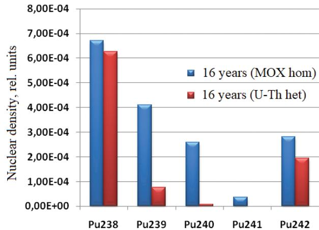
**Figure 3.** Plutonium nuclide contents in different transmutation options.
