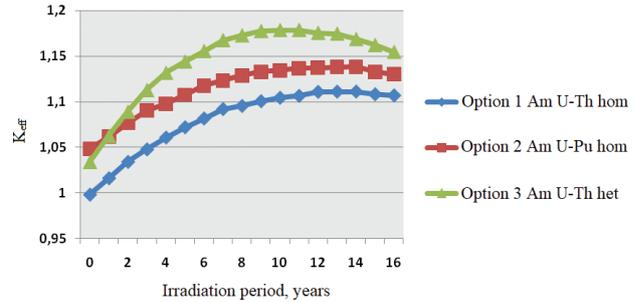
**Figure 2.** Change in  $K_{eff}$  depending on the duration of irradiation for the options of Am-reactors.
