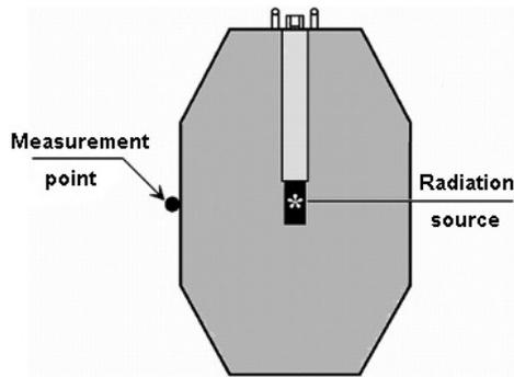
**Figure 2.** Measurement point and radiation source positions in the KL-15 cask.
