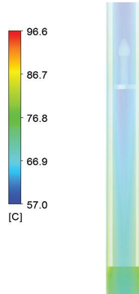
**Figure 5.** Temperature distribution through the coolant volume in the channel,  $^\circ\text{C}$  ( $90^\circ$  rotated).
