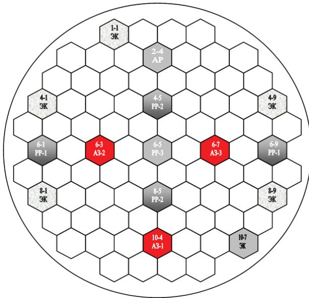
**Figure 1.** Layout of experimental channels for the  $^{99}\text{Mo}$  production (ECs 4-1, 4-9, 8-1, and 8-9) in the VVR-ts reactor core (Website of JSC All-Regional Association Izotop).
