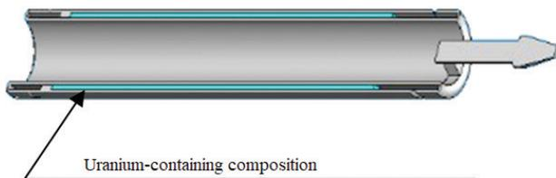
**Figure 3.** Diagram of a container unit for the  $^{99}\text{Mo}$  generation ( $90^\circ$  rotated).
