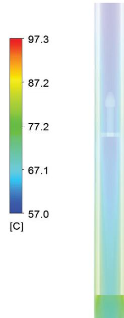
**Figure 6.** Temperature distribution through the coolant volume in the channel,  $^\circ\text{C}$  ( $90^\circ$  rotated).
