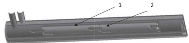
**Figure 4.** Diagram of the MAK-2 system with installed container units: 1 – upper target; 2 – lower target ( $90^\circ$  rotated diagram).
