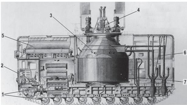
**Figure 4.** Scheme of the self-propelled vehicle with a reactor and service systems: 1. Self-propelled platform; 2. Body; 3. Reactor with shielding; 4. CPS actuators; 5. Radiator; 6. Pipeline of the primary circuit; 7. Technical water pipeline.
