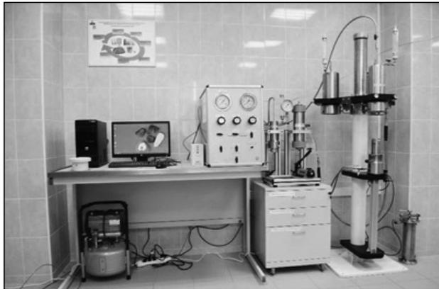
**Fig. 3.** UIP-ATM.002 training and research permeameter
