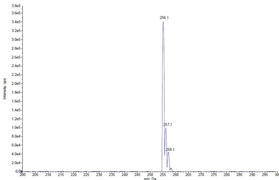
**Figure 2.** ESI<sup>+</sup>-mass spectrum of **VPZ**. **Note:** Mass-selective quadrupole detector AB Sciex QTrap 3200 MD; detection conditions – positive polarization ( $[M + H]^+$ ), electrospray ionization, electrospray voltage 5500.0 V, declustering potential 41.0; curtain gas pressure 20.0 psi, atomization gas pressure 40.0 psi, input potential 3.5 V. Solvent: acetonitrile: deionized water 2 : 1 with 0.1% formic acid. **VPZ** – **N-(5-ethyl-1,3,4-thiadiazole-2-yl)-2-propylpentanamide**.
