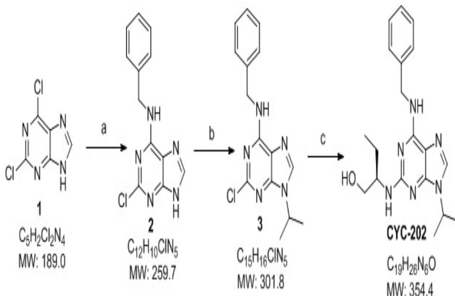
**Figure 4. Synthesis of CYC-202 ((*R*)-Roscovitine). Reagents and conditions: (a) benzylamine, BuOH,  $NEt_3$ ,  $110^\circ C$ , 3 h, 95%; (b) 2-bromopropane,  $K_2CO_3$ , DMSO,  $18-20^\circ C$ , 5 h, 85%; and (c) (*R*)-2-aminobutan-1-ol,  $160^\circ C$ , 8 h, 89%.**
