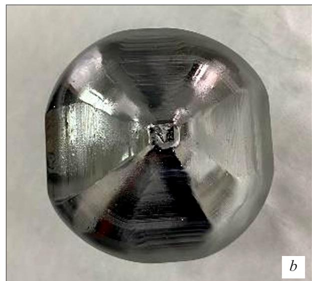
**Figure 4.** Appearance of indium antimonide single crystal: (a) 105 mm diam. single crystal and (b) facets of [100] single crystal.
